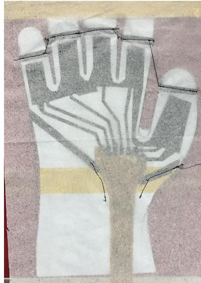
Sewing textile strips onto the Glove textile
